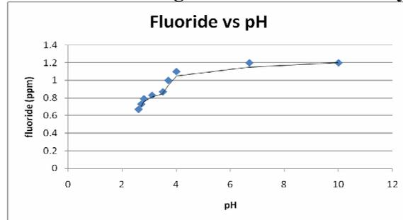
All readings were from a LaMotte fluoride specific electrode (calibrated with a 1.00 ppm sodium fluoride standard solution in distilled deionized water at room temperature). Readings for the 1.2 ppm true concentration solution in distilled water progressively decrease as pH decreases. Acidity was adjusted with dilute acetic acid. At stomach acid pH readings the fluoride is about 50% protonated, as hydrofluoric acid HF, and 50% free fluoride.
